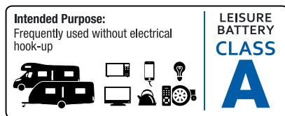
For motorhomes with higher power consumption but still generally used without electrical hook-up it may be more practical to use multiple batteries from class A to provide the required storage capacity than to specify a single battery of the required capacity.
