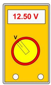
REMOVE FROM STOCK & RECHARGE ANY BATTERY THAT HAS REACHED THE SCHEDULED RECHARGE DATE OR IS FOUND TO HAVE AN OCV OF 12.50 VOLTS OR LESS
